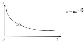
This is variation of displacement with time. This kind of motion is called **over-damped motion**.
