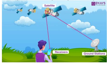
GPS is a system and it is made up of three parts: *satellites, ground stations,* and *receivers*.
