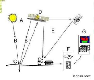
Source of Illumination (A) - provides electromagnetic energy to the target of interest.
