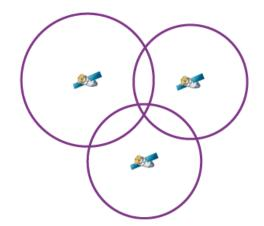
Trilateration is defined as the process of determining the location based on the intersections of the spheres. The distance between the satellite and the receiver is calculated by considering a 3-D sphere such that the satellite is located at the centre of the sphere. Using the same method, the distance for all the 3 GPS satellites from the receiver is calculated.
